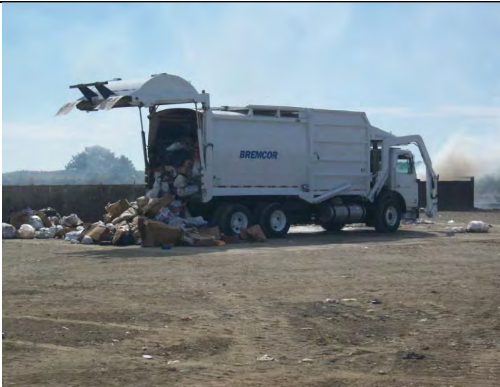
Photograph: 3 Collection truck discharging load for sampling Solid Waste Characterization Study Naval Station Guantanamo Bay (GTMO), Cuba
