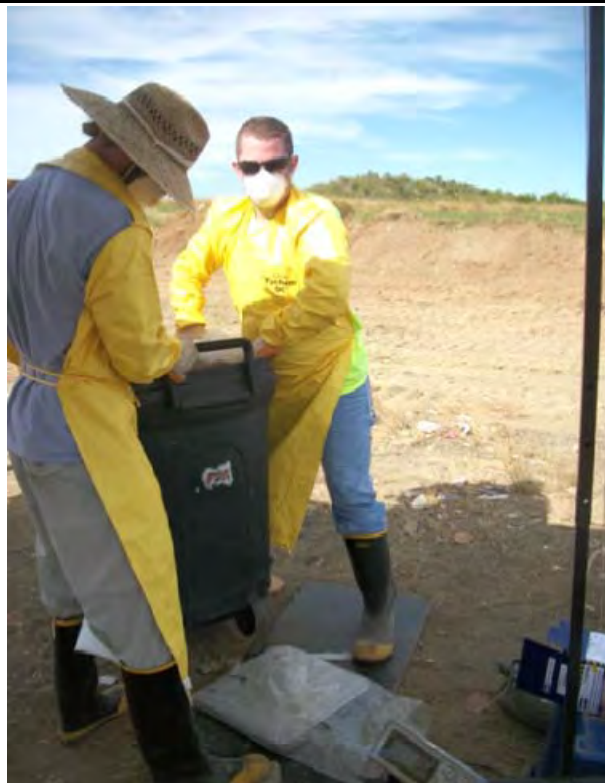
Photograph: 6 Weighing sample and transporting from tarp to clean plywood sorting table Solid Waste Characterization Study Naval Station Guantanamo Bay (GTMO), Cuba
