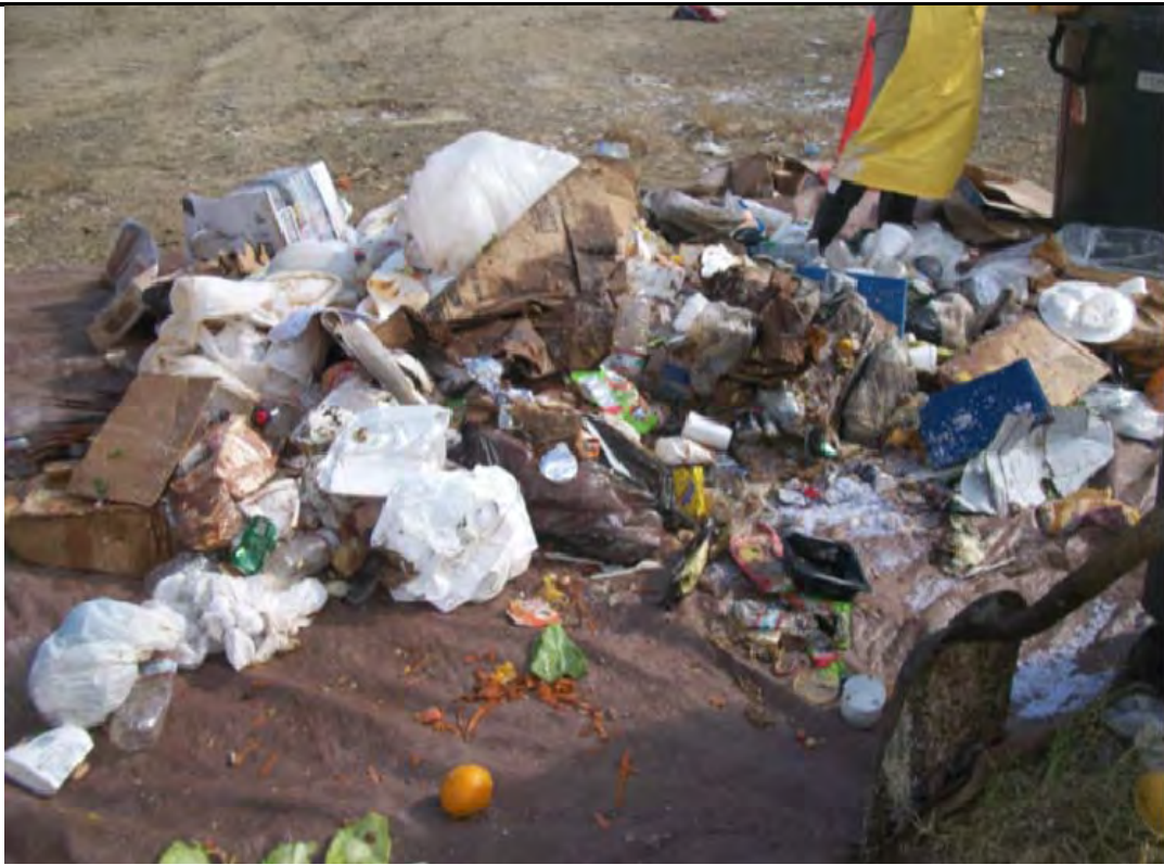
Photograph: 5 Sample on tarp Solid Waste Characterization Study Naval Station Guantanamo Bay (GTMO), Cuba
