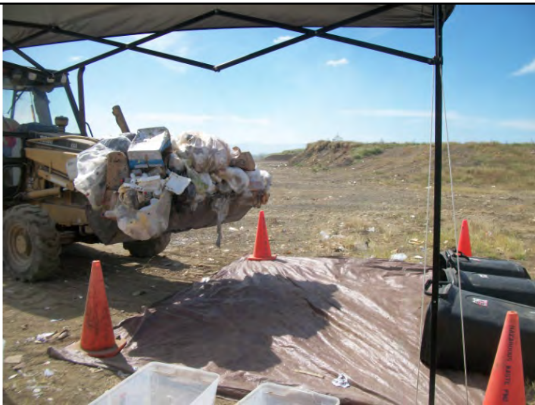
Photograph: 4 Front-end loader transporting sample to clean tarp Solid Waste Characterization Study Naval Station Guantanamo Bay (GTMO), Cuba
