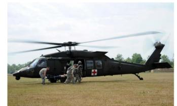
**HH-60M "Blackhawk"** The HH-60M "Blackhawk" is designed for MEDEVAC missions and is equipped to provide en-route medical care for patients being transported from an injury site to a hospital facility. This rotary-wing aircraft includes an environmental control system, oxygen-generating system, patient monitors, and an external electrical rescue hoist.
