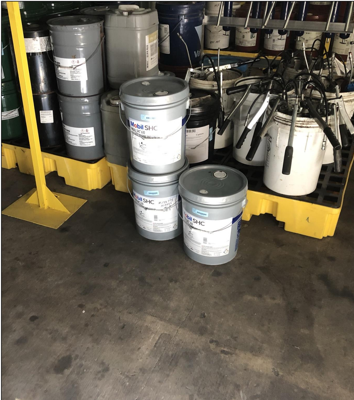
HM/HW containers stored without secondary containment in Building 158 (storm drains located inside building).
