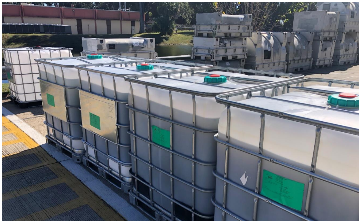
Multiple totes of engine washing wastewater stored outside Building 797 without secondary containment.
