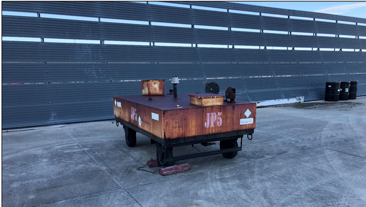
Heavily rusted fuel cart located on the west end of Hangar 511.
