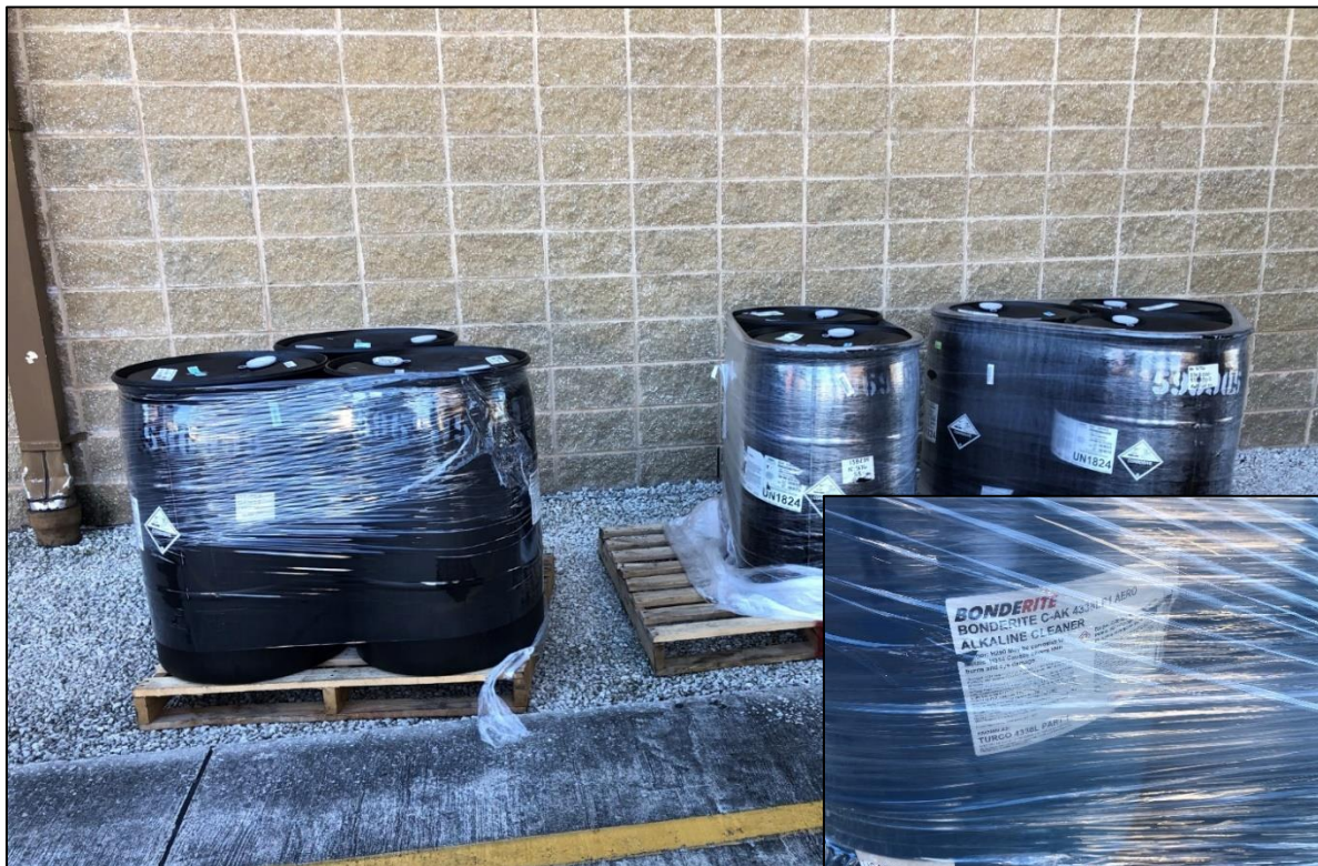
Multiple drums of cleaner stored outside Building 794 without secondary containment.
