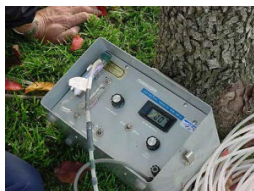
Fumigator for monitoring fumigant gas in structure
